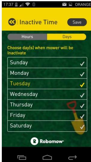
The Days settings define the days in a week when Robomow is not allowed to leave the base (i.e., remains inactive). By default, Sunday is set as an inactive day. To make a particular day inactive, select it in the list. A day displayed in yellow is an inactive day. A day displayed in gray is an active day.
